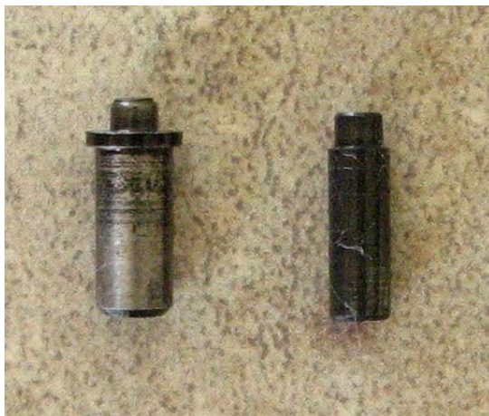
Wartime (left) and post-war (right) firing pin retaining pins.
