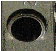
Wartime firing pin retaining pin hole (as seen from the top of the slide).
